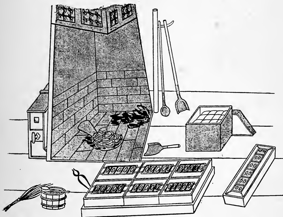
Fig. 8.—FURNACE AND MOULDS USED IN MELTING AND CASTING SILVER.
